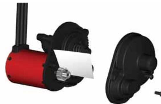
To set the gear mesh, screw the motor into the corresponding marked set of holes. For example, with a 20T pinion, the motor screws must be screwed into the holes labeled “20”.
